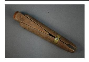
Wood wedge to tighten ring clamp (Part a).
